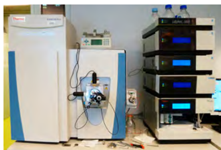
Fig. 2: Nano-LC-MS system consisting of a Q Exactive™ Hybrid Quadrupole-Orbitrap Mass Spectrometer (Thermo Scientific™) and a nano-LC gradient system UltiMate 3000 (Dionex).
