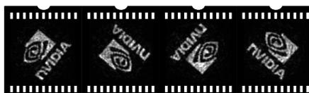
Pattern, consisting of 4000 points and generated in real-time, displayed at the output facet of the multimode fiber
