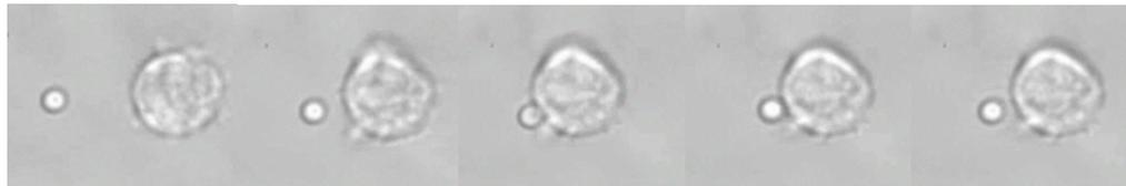
Frames showing (left to right) acquisition of trap stiffness, approach to cell, bead-cell contact, applying a pulling force to the bead, and integrin-ligand bond breaking, resulting in the bead jumping back in to the trap.
