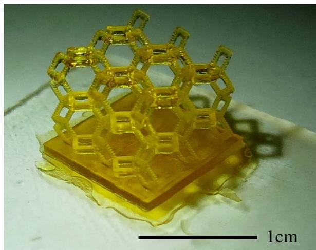
Figure: high resolution 3D printed lattice structure created by our printer.
